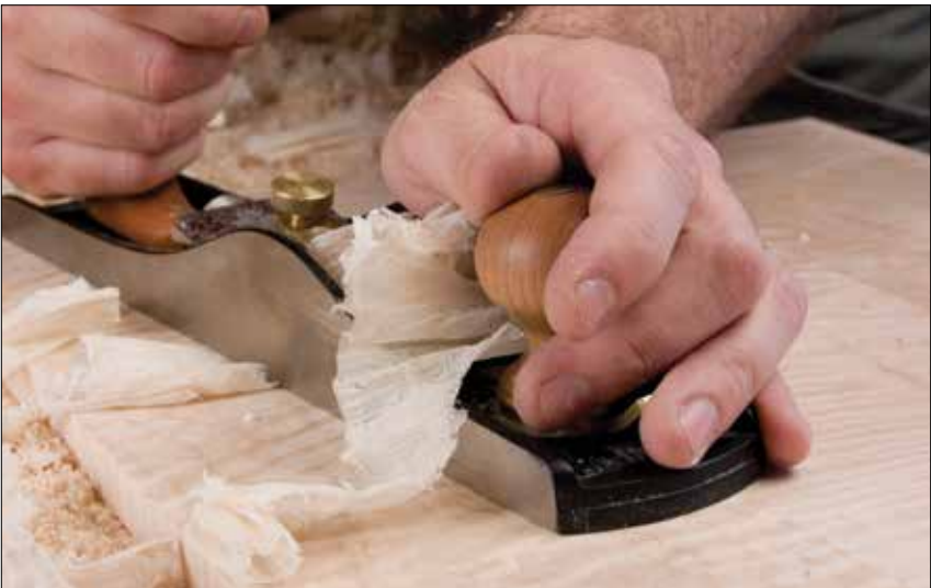
Last, a few passes with a finely-set blade and tight mouth yields a glass-smooth, ready to finish surface.
