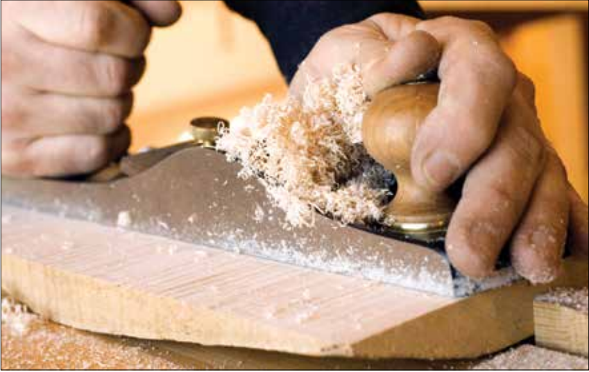
First, use a toothed blade for heavy stock removal.
