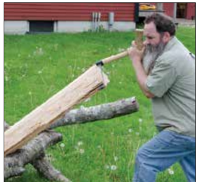
(Above) Master Joiner, Peter Follansbee, rives stock with the Langsner Froe in our video, "17th Century Joined Chest" (p. 70).
