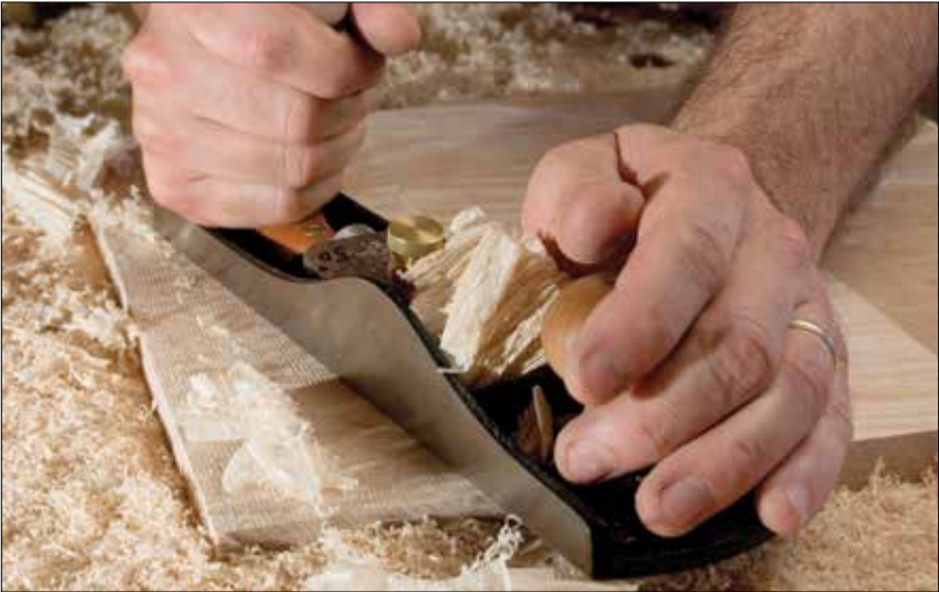
Second, use a 50° micro-beveled blade and medium mouth opening to remove tothing marks.
