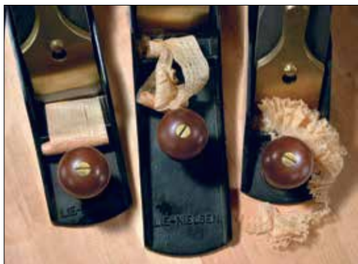
(From left to right) Coarse, Medium, and Fine shavings
